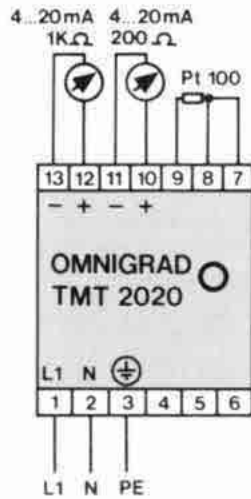
Fig. 4 TMT 2020 electrical connections.
